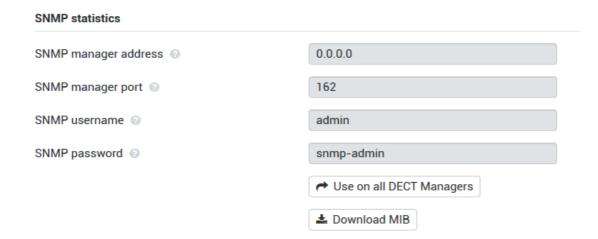
▶ Enter the IP address of the SNMP manager server in the **SNMP manager address** field and the port number used by the SNMP manager in the **SNMP manager port** field. Default: 162
